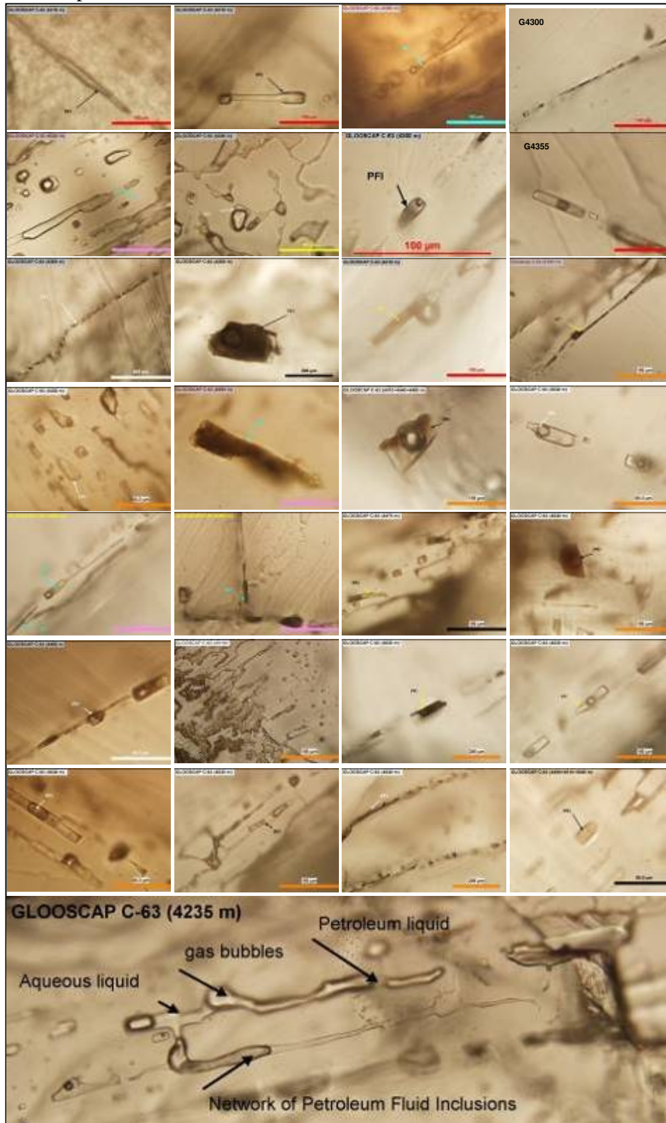
Fig. 10: Various shapes of petroleum-bearing fluid inclusions in Argo Salt at the Glooscap-C63 well.
