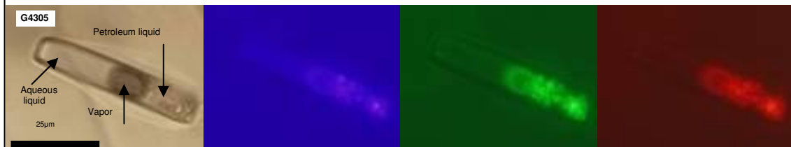
Four-phased (petroleum liquid + aqueous liquid + impurities + vapor or gas bubble) FI
