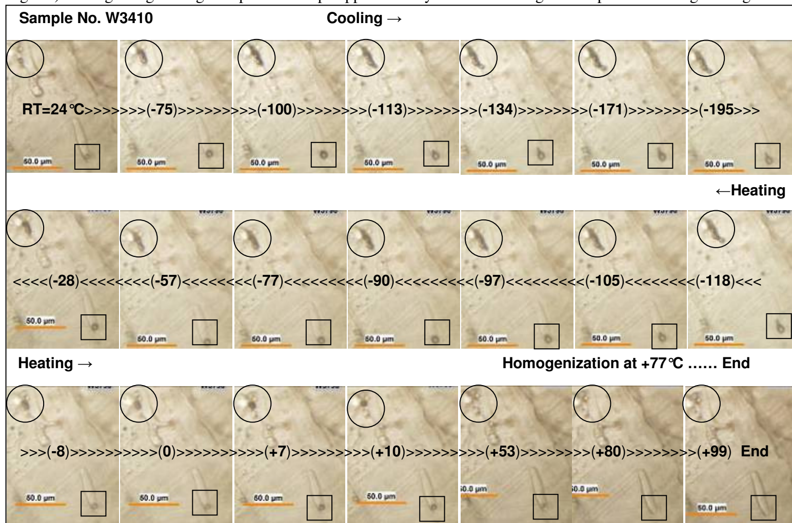
Fig. 44b: Microthermometric treatment of two-phased liquid petroleum inclusions (PFI) which neither showed any color changes nor distinct signs during phase changes other than gradual size increase and deformation of the bubble during cooling ( \sim > -75^{\circ}\text{C} \pm \text{few degrees} ) and regaining its original spherical shape approximately at the same range of temperature during heating.
